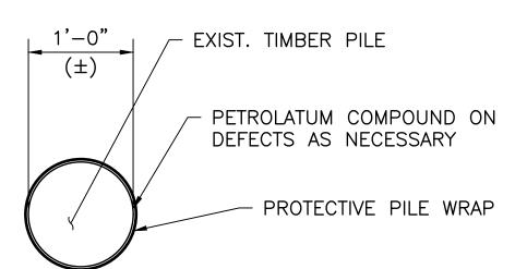
F CROSS SECTION OF PILE WITH WRAP
