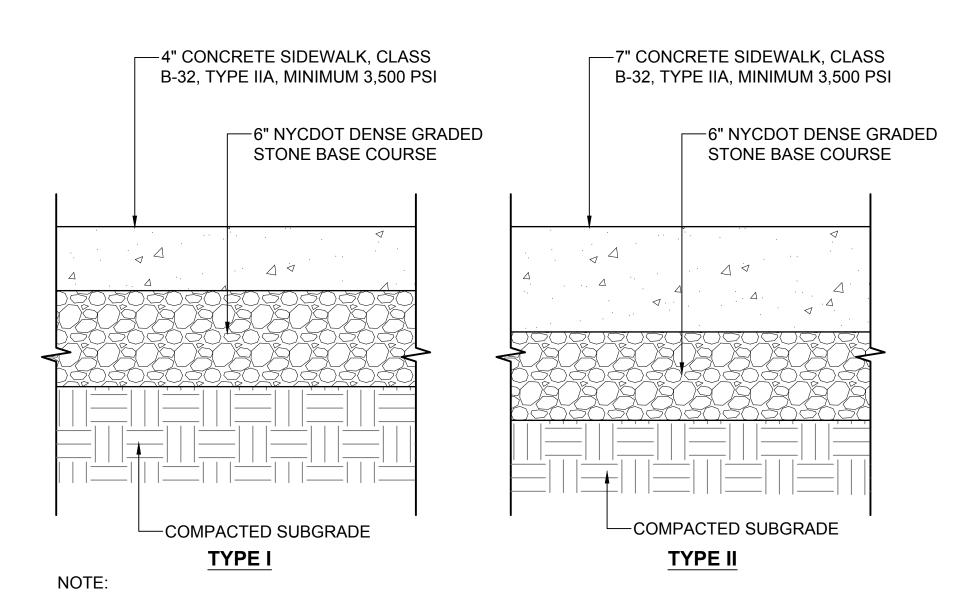
1. ALL MATERIALS AND CONSTRUCTION METHODS USED ARE TO CONFORM TO SECTION #4.13 OF THE LATEST NYC DEPARTMENT OF TRANSPORTATION (DOT) STANDARD HIGHWAY SPECIFICATIONS AND STANDARD DETAIL H-1045.
