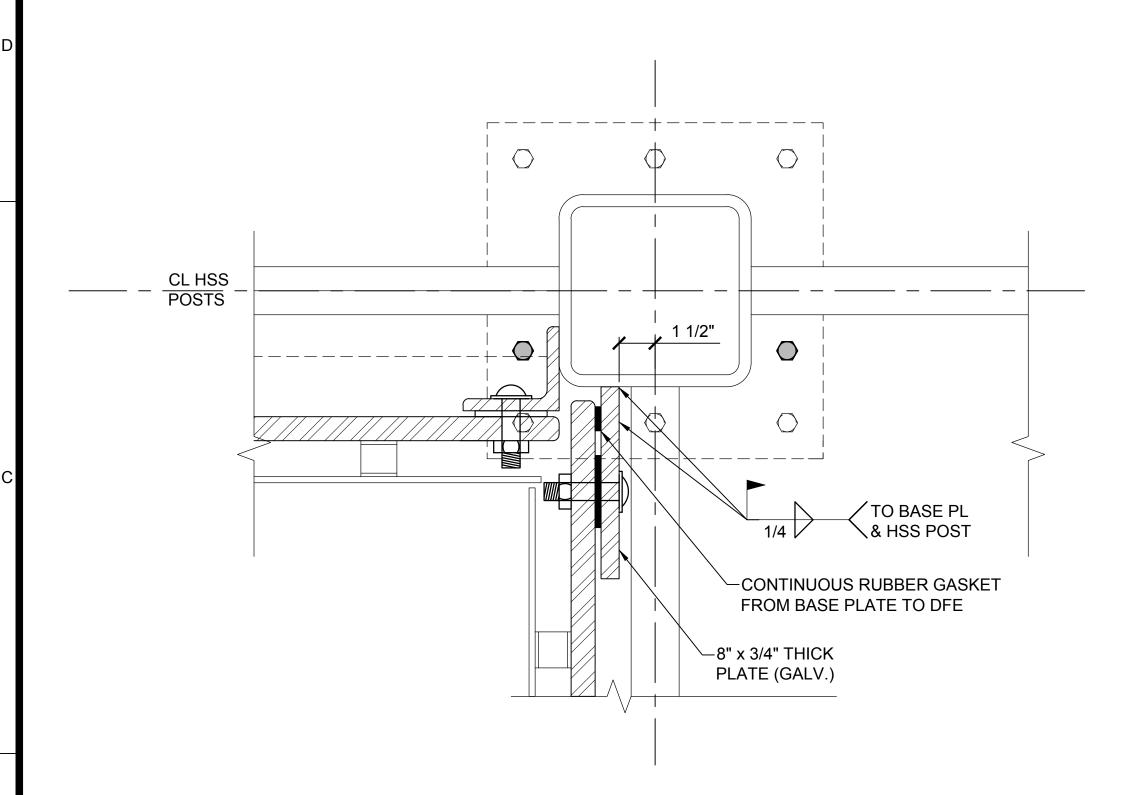
STEEL PLATE FLOOD WALL CORNER DETAIL
