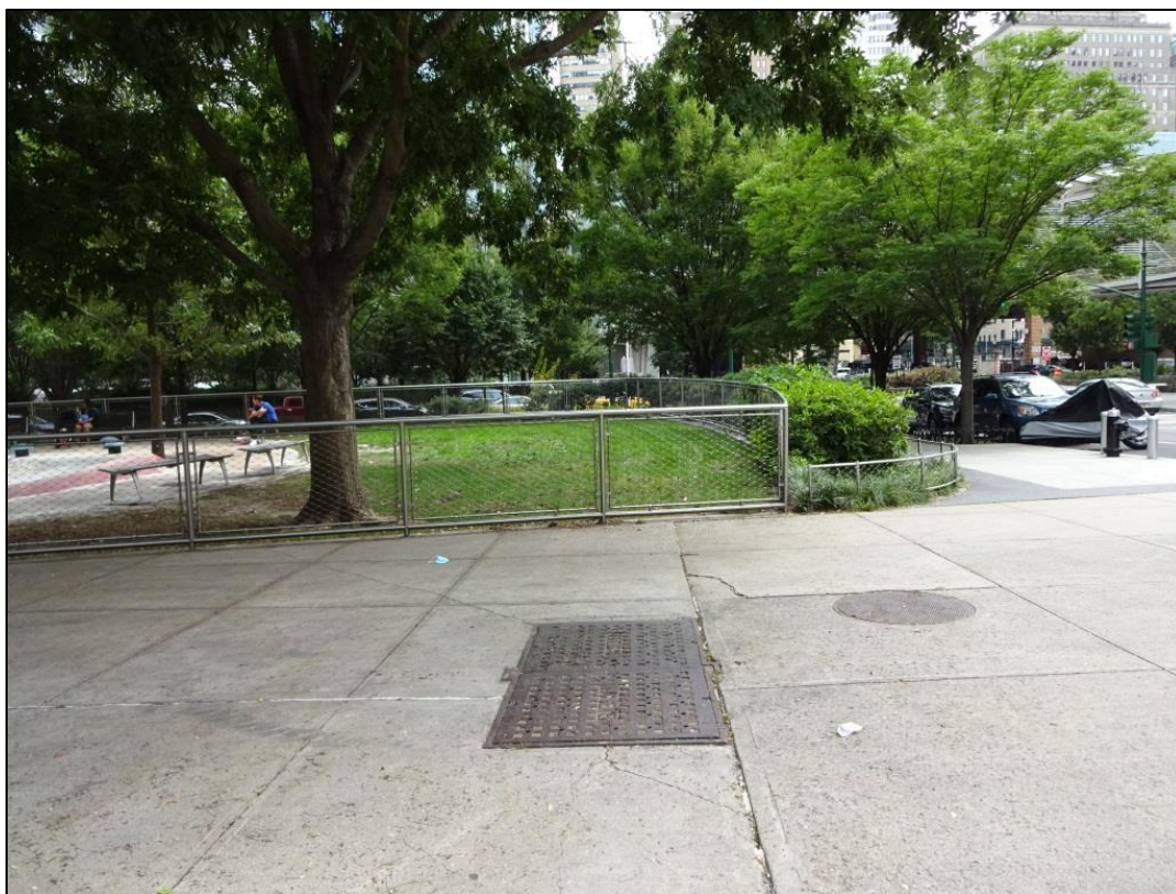
Looking east toward existing sanitary emergency overflow chamber; as part of the NSI improvements, the manhole cover would be replaced with a pressure-proofed opening.
