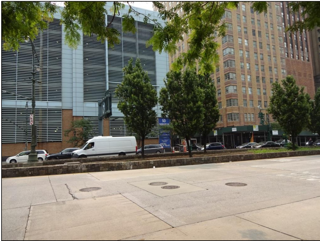
View looking east toward West Street (Route 9A) and manholes associated with Regulator M8. Note 21 West Street and Downtown Athletic Club at right edge of photograph. NSI improvements would be made in this area, including replacement of manhole covers with pressure-proofed openings.
