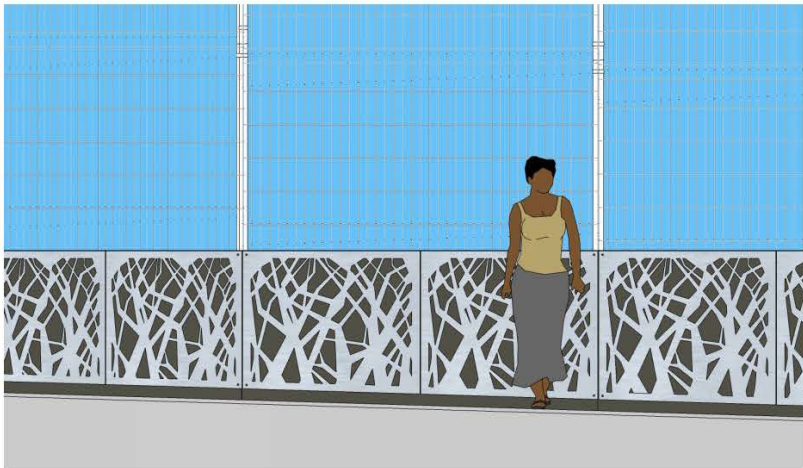
PANELS MAINTAIN 3' MIN. HEIGHT AS FLOODWALL TAPERS STEEL FLOODWALL FINISH: SHERWIN WILLIAMS SEALSKIN #7675 HIGH PERFORMANCE MICA FINISH ARCHITECTURAL PANEL FINISH: 6061 ALUMINUM WITH CLASS 1 CLEAR ANODIZATION
